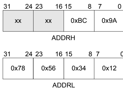
Figure 4.1 Example ADDRL, ADDRH Address Ordering
