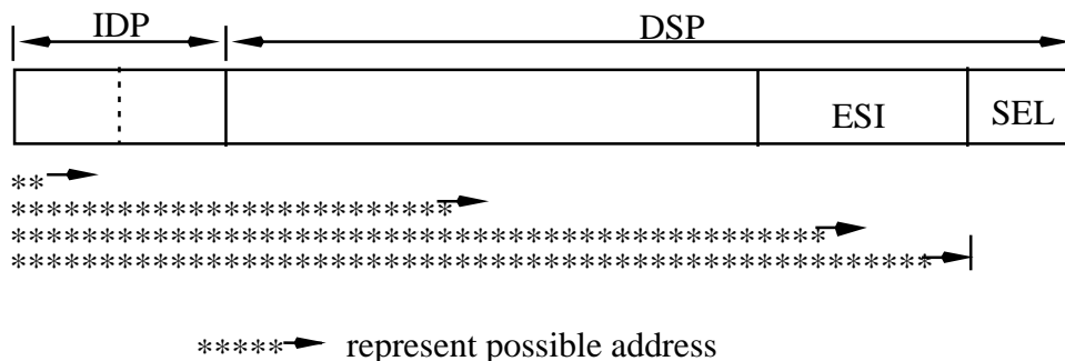
Figure 5-1: NSAP Address Structure and Address Prefixes
