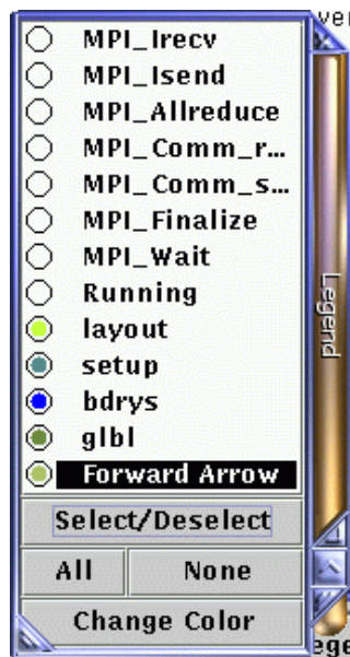
Figure 5: All MPI and OS-related states are deselected in the “Preview” and “Legend” to highlight the user-defined states and the communication among the processes.
